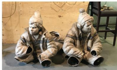
Raw and cleaned bronze components ready for surface finishing and assembly
