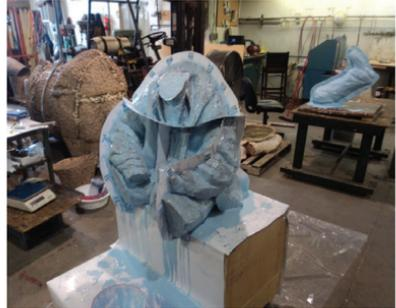
Painting on rubber mould material onto the clay model - preparing rubber moulds for wax model, 2017
